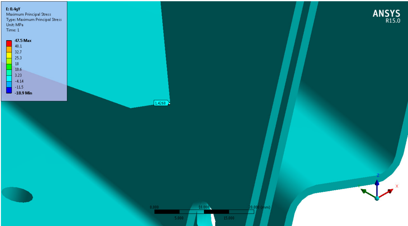
Figure 9_11 - GM/RT 2100 0.4gY Principal stress range - CDR type 1 installation, weld region
