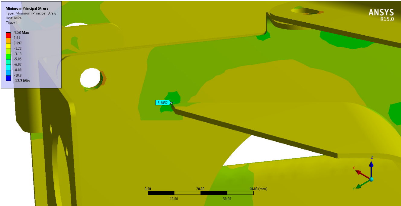
Figure 10_10 - GM/RT 2100 0.3gX Principal stress range - CDR type 2 installation, weld region
