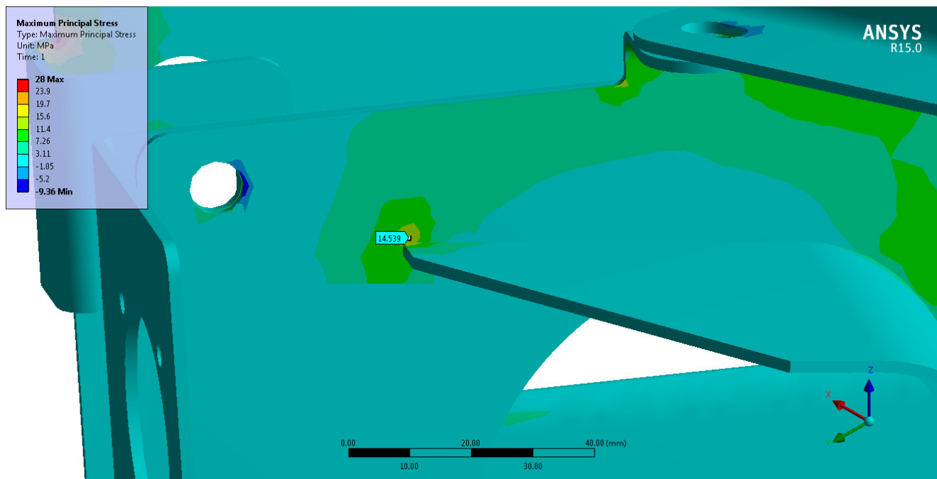
Figure 10_12 - GM/RT 2100 0.5gZ Principal stress range - CDR type 2 installation, weld region
