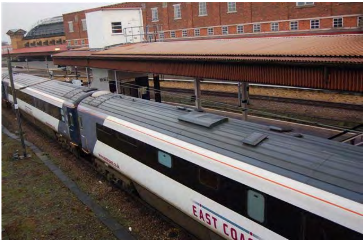
Figure 3: Catering Area Roof Cows on HST TBRF
