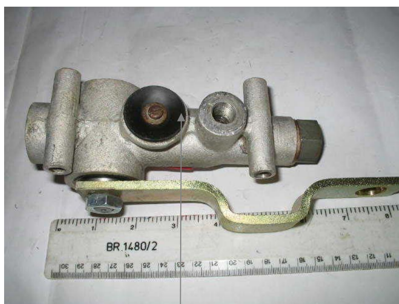
Figure 1: Cast Type Levelling Valve
