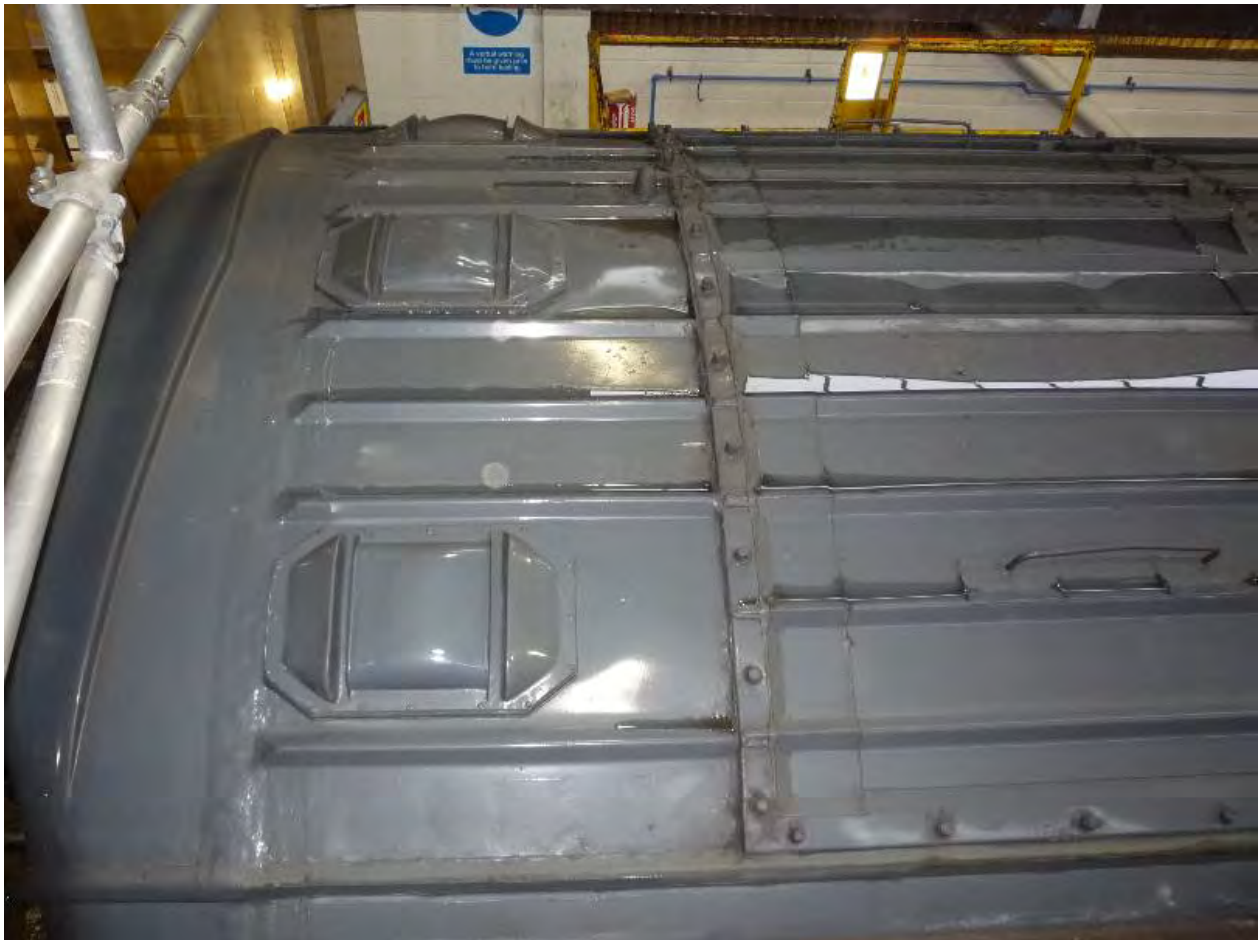
Figure 1: Three Roof End Ventilators Mk 3A (quantities/vehicles are confirmed more accurately in the text)
