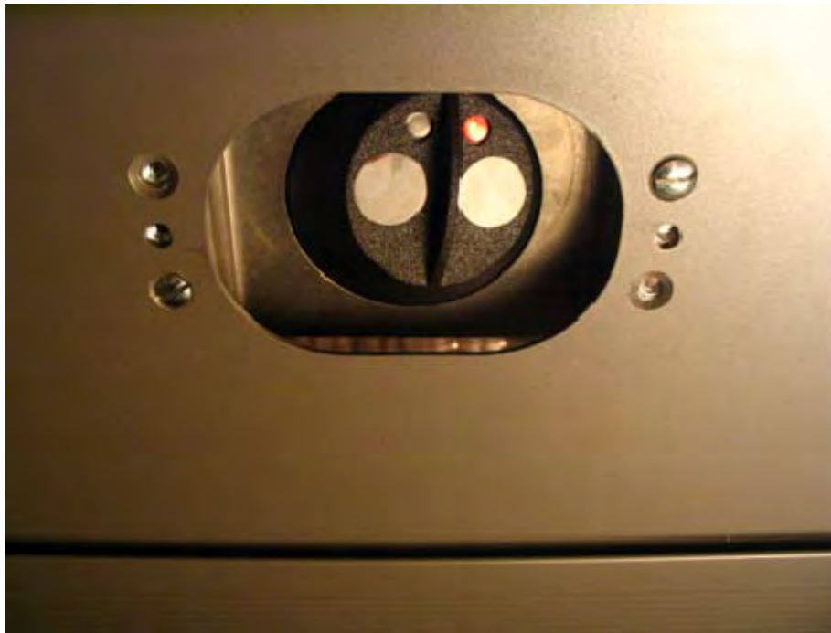
Figure 1: Ceiling Mounted PIR Sensor
