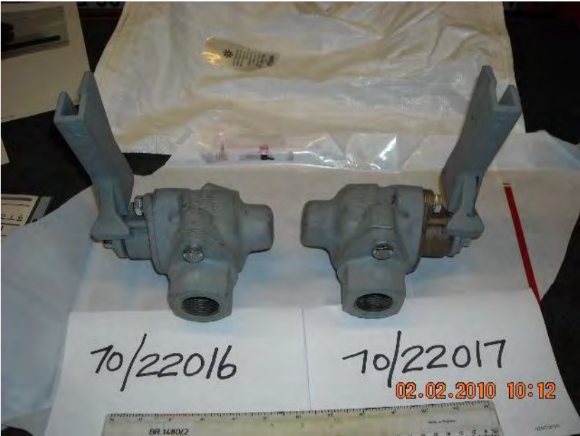
Figure 1: Identification of Coupling Cocks
