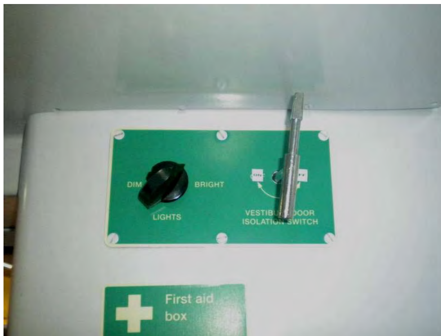
Figure 10: Door Isolation Switch
