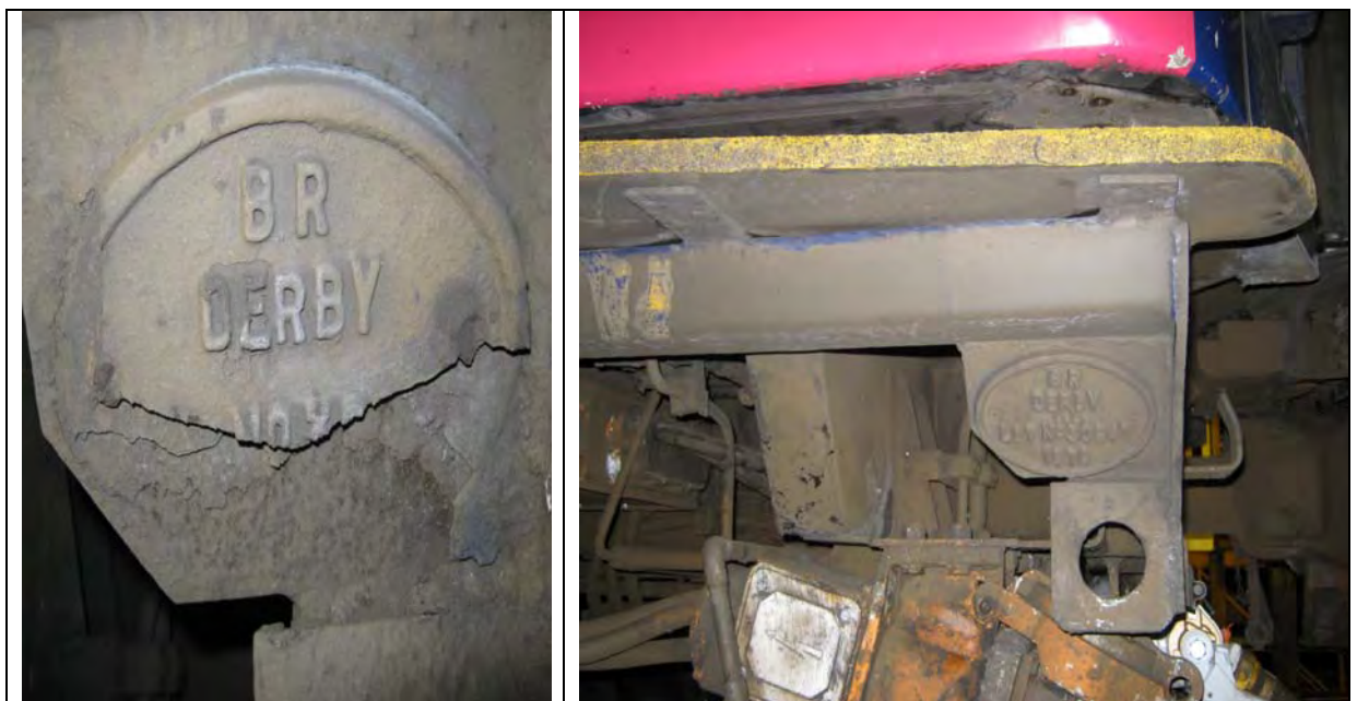
Figure 4: Example of Broken Builders Plate and Location
