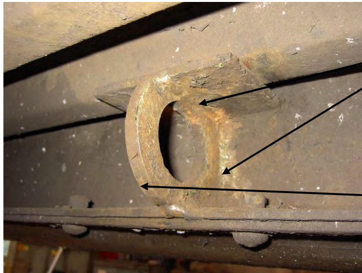
Figure 1: Measuring Loop Plate Thickness
