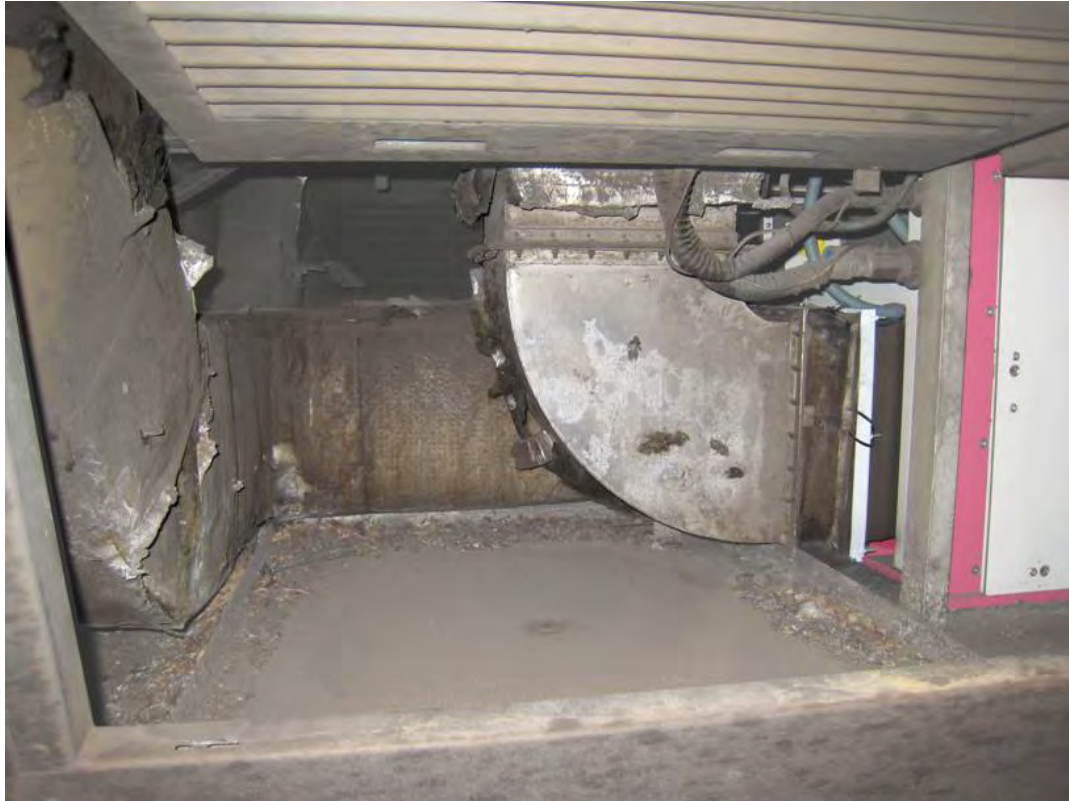
Figure 1: Typical View of Air Conditioning Fixed and Flexible Ducts in the Underskirt
