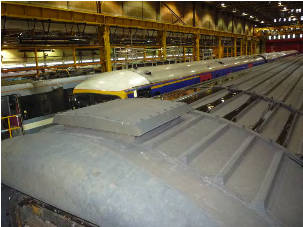
Figure 2: Roof End Cowl Mk 3B and HST (quantities/vehicles are confirmed more accurately in the text)
