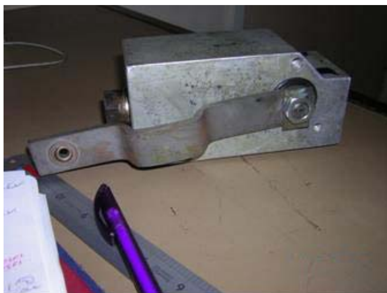
Figure 2: Block Type Levelling Valve with Cut Out
